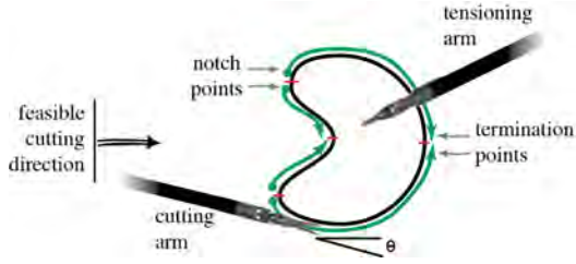
Fig. 3: The dVRK arms have limited approach angles, and cutting can only happen along a vector where the angle \theta from the forward direction from the base of the arm is less than or equal to 90 degrees in magnitude, with equality only permitted for isolated points. This requires segmenting contours into multiple sections for cutting. Notch and termination points are locations at the limits of the cutting arm’s range of motions, or those orthogonal to the main approach direction of the arm, and the direction of cutting is always in the main approach direction.
